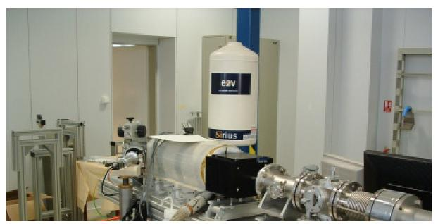
Fig. 1 This photo shows the terminal of the proton beam line with quadrupole magnets focussing the beam on the sandstone sample, beam scanner and the cooling system of the quadrupoles. The target chamber, positioned at the end of the proton beam line, was equipped with the X-ray Si(Li) and RBS detectors.
