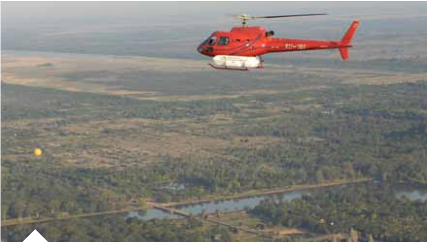
Helicopter with lidar attached during flight operations over Angkor, April 2012
