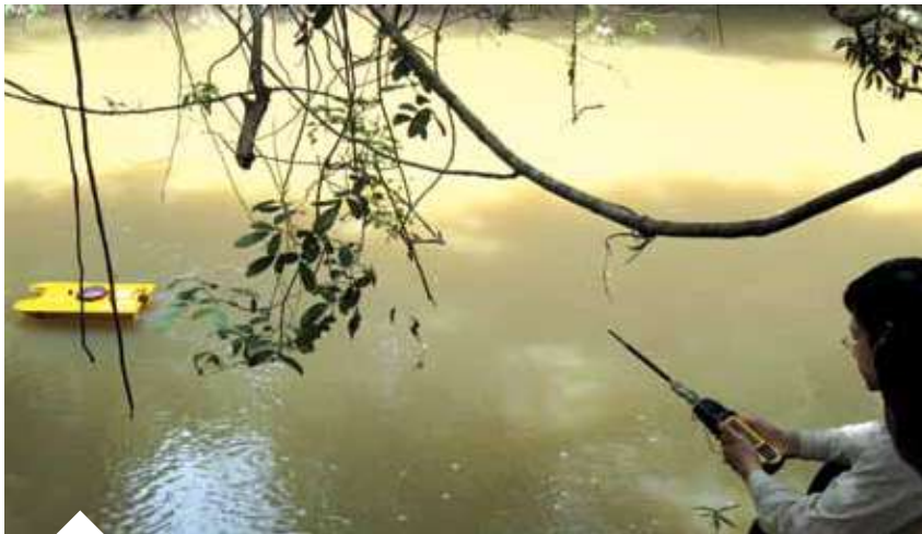
Measuring the flow of the river of Siem Reap with Qliner
