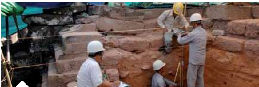
Penetration test on the foundation soil of the Southern Library
