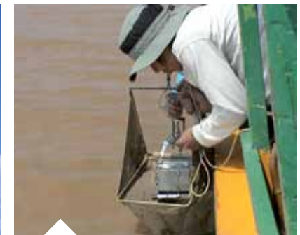
Benthic organisms sampling using an Ekman-Berge sampler - Tonle Sap Lake
