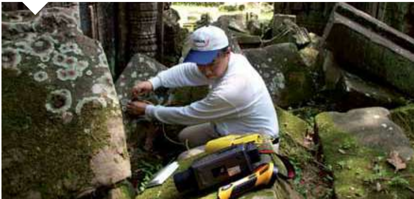
Measurement of the hardness of the stone and its microflora in a microclimate
