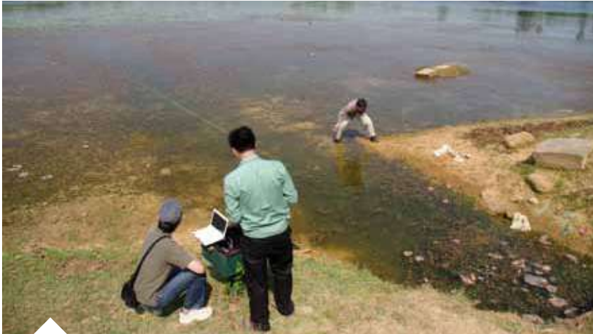
Installation of a precise water pressure logger in the Srah Srang reservoir
